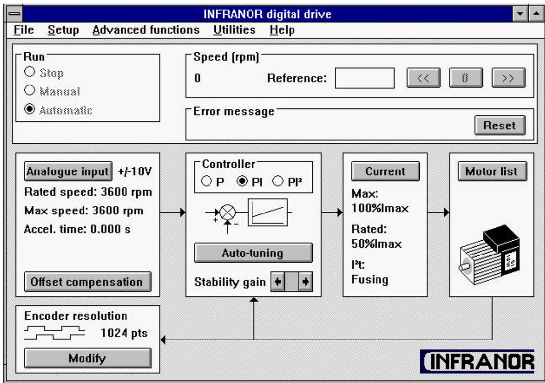
The INFRANOR Digital Drive graphic window has an adjustment panel, a control panel and functions accessible via menus. This presentation allows a quick adjustment of the system's main parameters during the commissioning and the adjustment phases.
