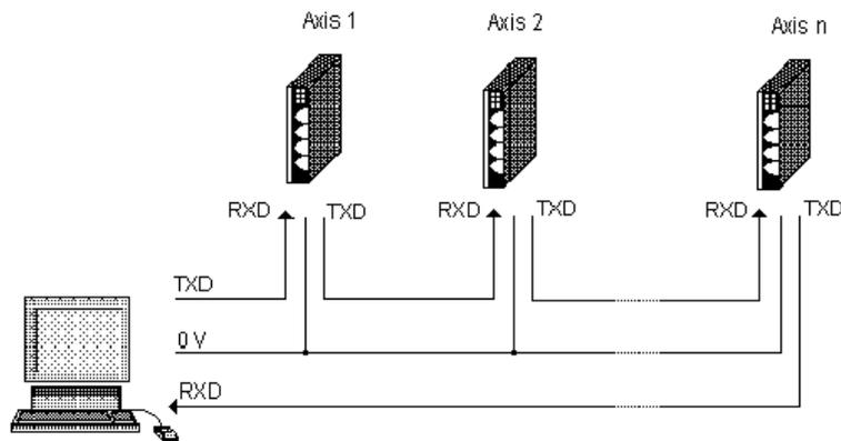
The connection of the various units (computer or amplifiers) is made as a ring: the transmission signal (TxD) of each unit is connected to the reception signal (RxD) of the next unit. Each amplifier has a software address (1...15) assigned which is stored into the EEPROM memory of the amplifier. The amplifiers on a ring must have different addresses.
