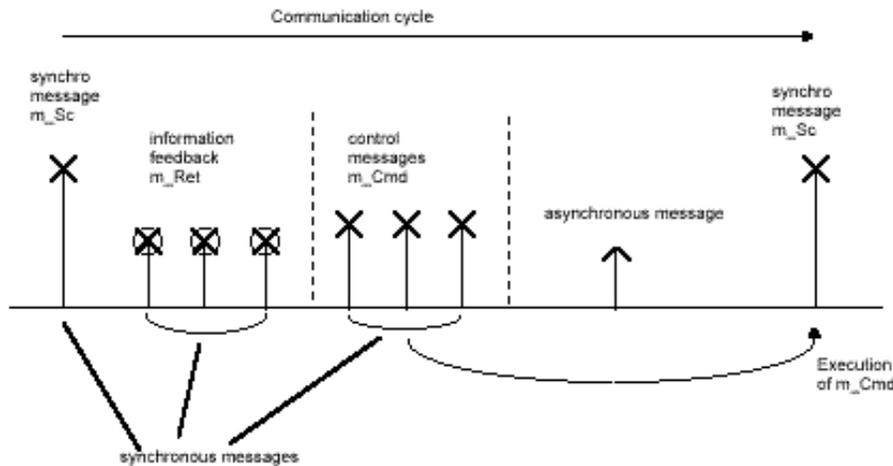
At constant time intervals (cycle time), the NC sends a synchro message m\_Sc and the amplifiers of the same synchronisation group acquire their position and send the messages containing their position (m\_Ret). After the reception of the positions, the NC sends the input command messages (m\_Cmd) to the amplifiers of this same synchro group.
