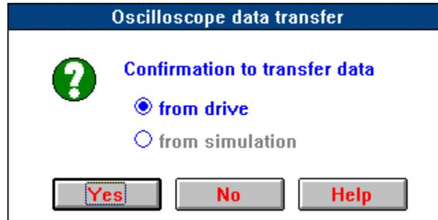
The transfer from the amplifier (**Transfer from drive**) is only possible when the amplifier is in use. The transfer time is depending on the communication speed and on the number of selected curves. Transfer time at 4800 baud: about 12 s per curve.
