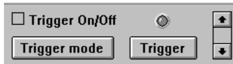
**Trigger On/Off** allows to cancel or display the triggering level cursor on the oscilloscope screen (in red).
