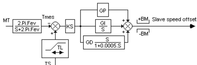
**Tension loop adjustment** submenu in the **Advanced functions** menu of the BPCW software allows the access to all regulator parameters.
