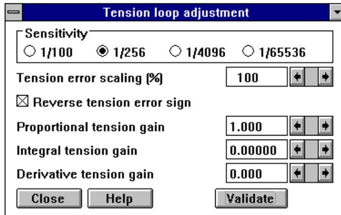
**Tension error scaling** defines the reduction factor **KS** acting on the tension error in order to adjust the tension regulator gains to the application specifications. The adjustment range is between 10 % and 100 %.
