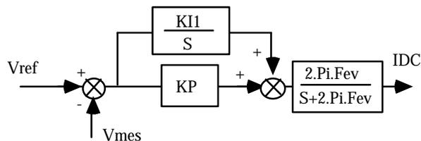
The gain parameters are automatically calculated during the **AUTOTUNING** procedure and are accessible via the submenu **Controller parameters** of the menu **Advanced Functions**.
