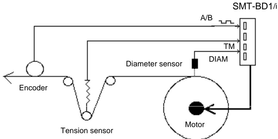
The rotation speed of the empty spool is defined by the ratio between the line encoder resolution and the motor resolution (Empty spool speed = Line encoder speed x Line encoder resolution / Motor resolution). The motor encoder resolution is programmable between 1 and 8192 ppr. The maximum motor rotation speed (corresponding to the empty spool) is adjustable between 100 rpm and 14000 rpm.
