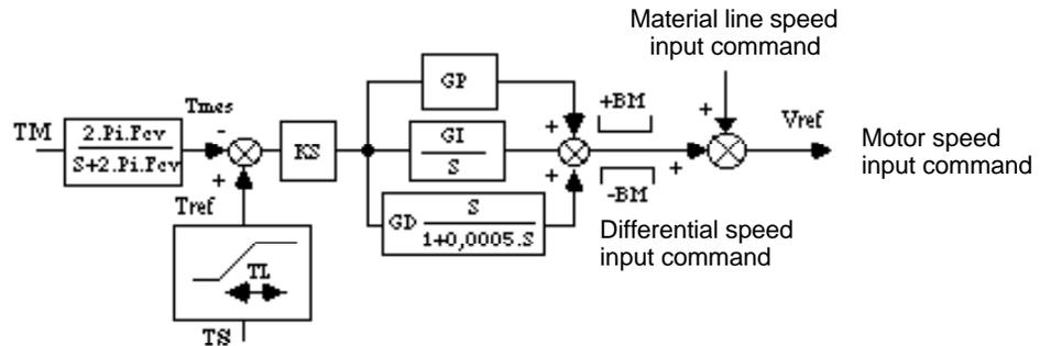
The gain parameters of the tension regulator are accessible in the submenu **Tension loop adjustment** of the menu **Advanced Functions** of the BPCW software:
