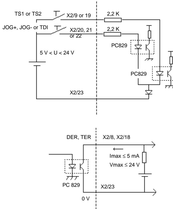
The **DER** and **TER** outputs (error indication) are "open collector" and "optocoupled". The transistor is inhibited when a default occurs. The application scheme is shown below. The maximum output current is 5 mA.
