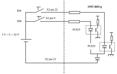
The POS and REG outputs are "open collector" and "optocoupled" outputs. The transistor is open if a fault occurs. The traditional application scheme is shown below. The maximum output current is 5 mA.
