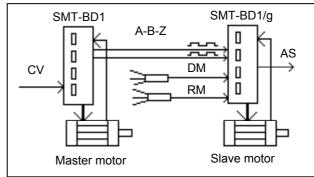
The photocell connected to the **DM** input of the amplifier **X2** connector allows the detection of the master axis reference positions. The photocell connected to the **RM** input of the **X2** connector allows the position detection of the products to be registered for the position interval calculation. The **AS** analog output of the amplifier **X4** connector provides a motor speed monitor sized between +/- 10 V.
