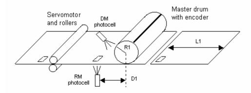
In this case, the registration control allows to compensate the material slippages and the interval variations between the registration marks, in order to keep the drum position always aligned on the synchronization marks.
