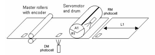
In this case, drum and material must be synchronized for a given distance according to the material registration marks and the drum photocell position.
