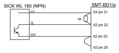
Connection of an PNP photocell with use of the + 15 V amplifier supply.
